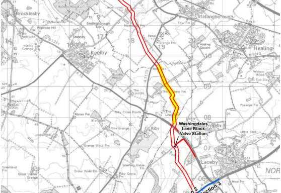
2.6 The pipeline will be designed for a minimum operational life of 25 years. The pipeline is expected to have an external diameter of 24" (609 mm) and be buried to a minimum depth of 1.2 m to the top of the pipe. This will be greater at crossing points of railways, roads and watercourses.
